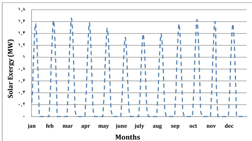
Figure 15 The solar exergy amount added to the system
