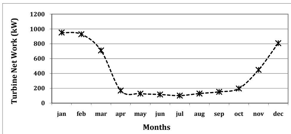
Figure 12 The monthly average producible net work by the turbo expander
