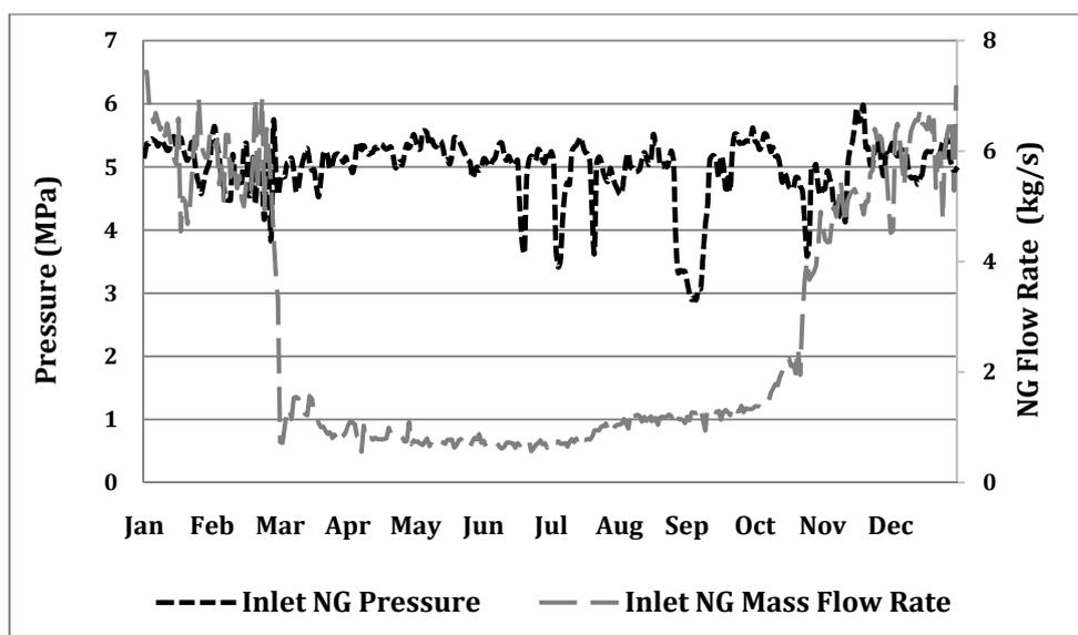
Figure 6 Natural gas pressure and mass flow rate in 2011
