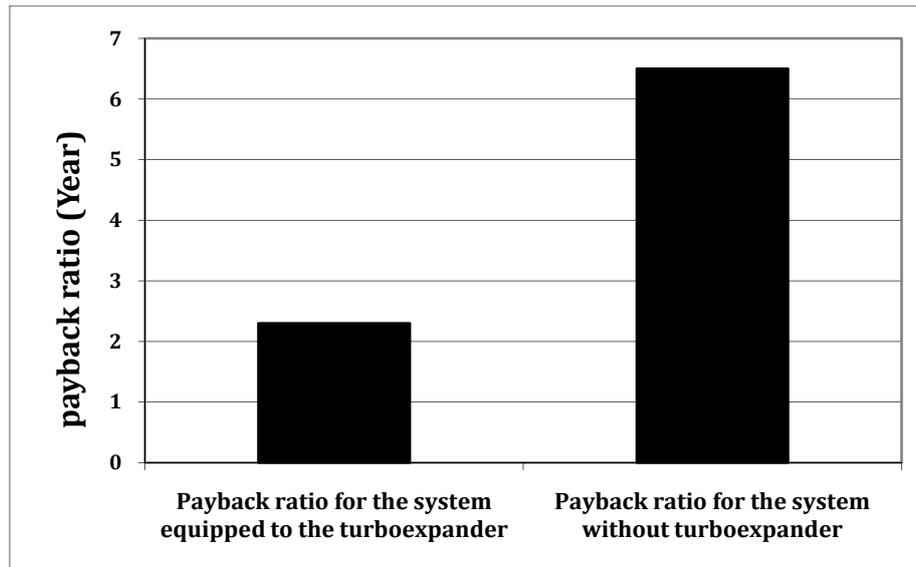
Figure 13 Simple payback ration comparison
