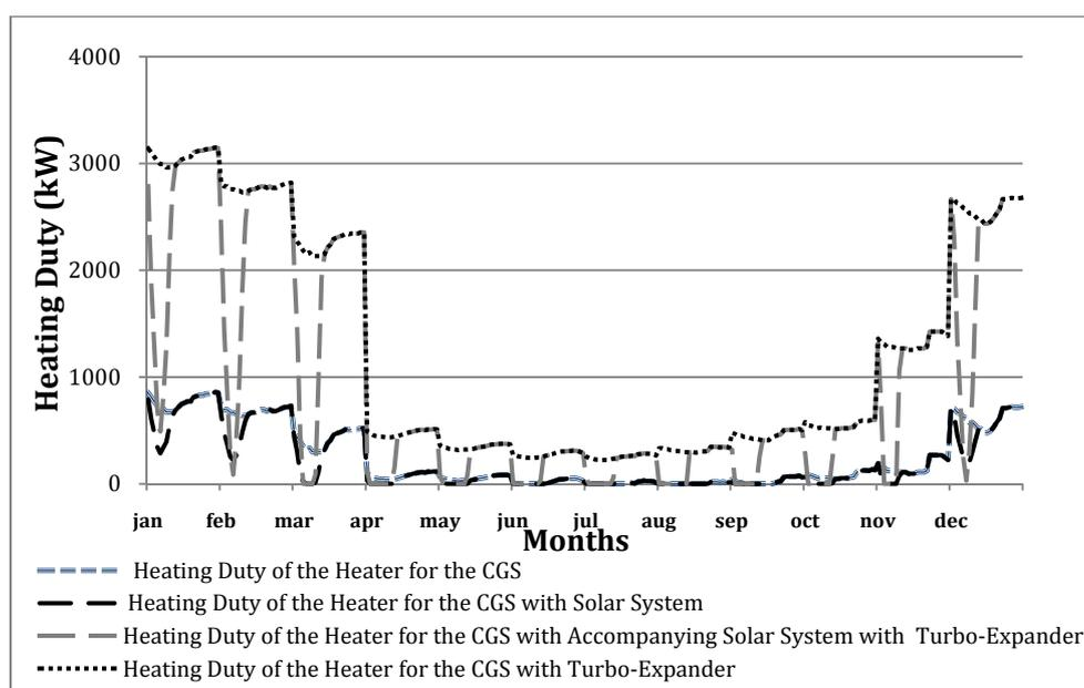
**Figure 8** Comparison between monthly and hourly average heating duty of the heater for four different cases
