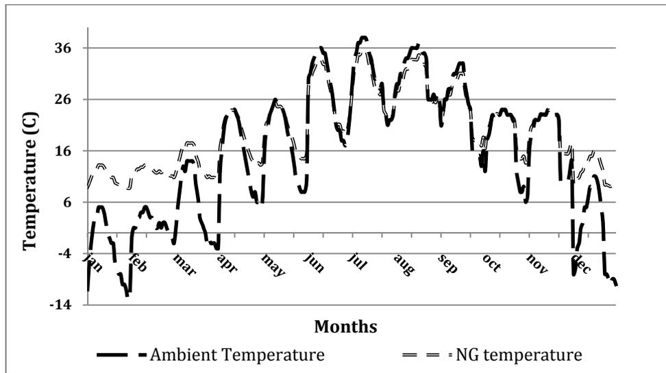
Figure 5 Birjand ambient and CGS inlet gas temperatures in 2011
