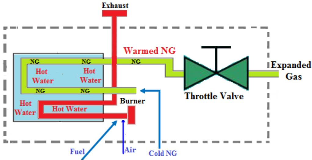
**Figure 3** The conventional configuration control volume details
