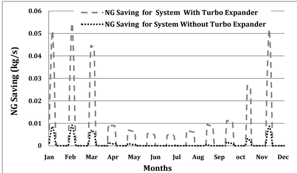
Figure 9 Fuel saving in with/without turbo expander systems
