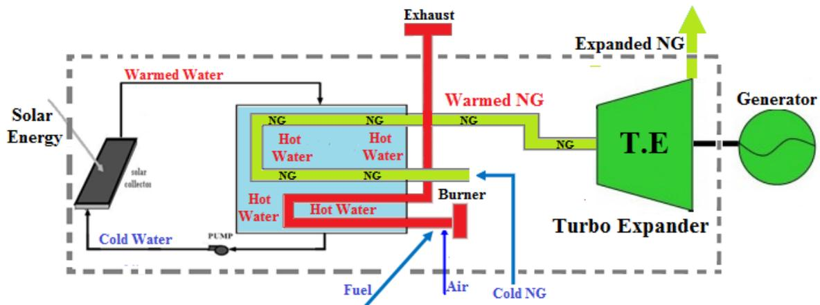
Figure 4 The improved configuration control volume
