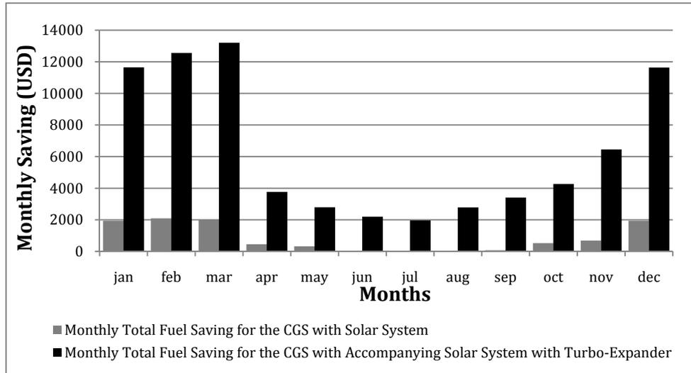
Figure 11 Total monthly fuel saving for both with/without electricity generator system in 2011
