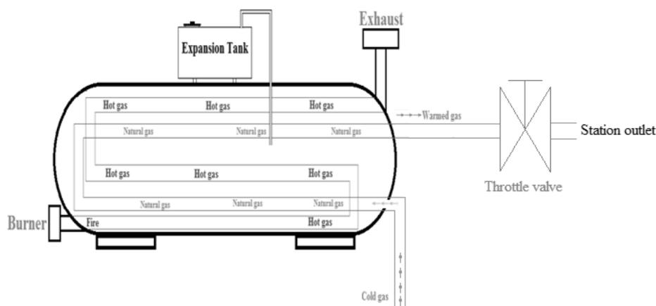
**Figure 1** Schematic diagram of a natural gas pressure reduction station
