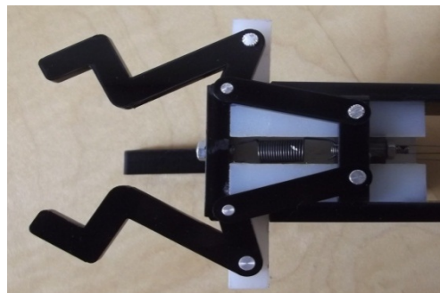
Figure 7 The spring embedded into the groove.
