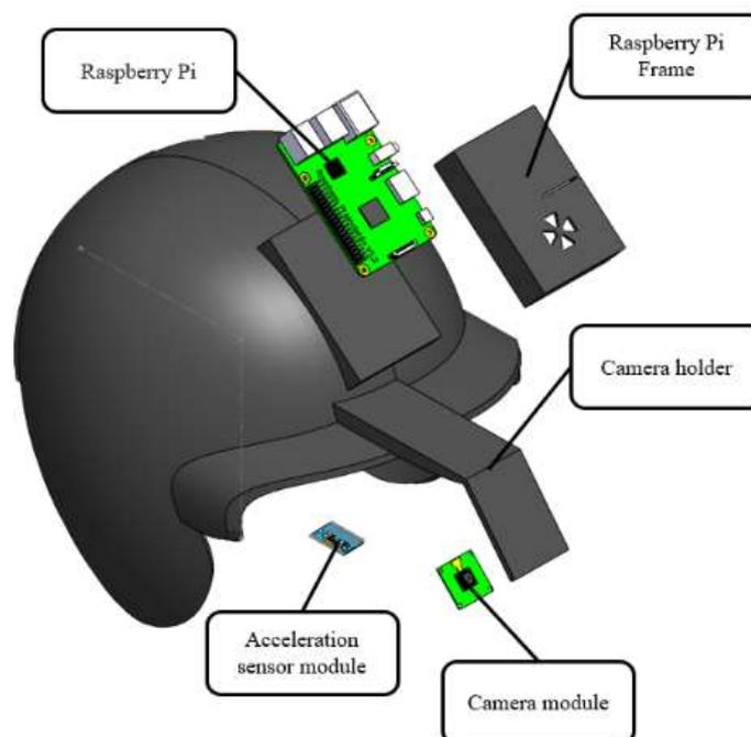
Figure 5 Explosive view of wearable motion control interface gadget
