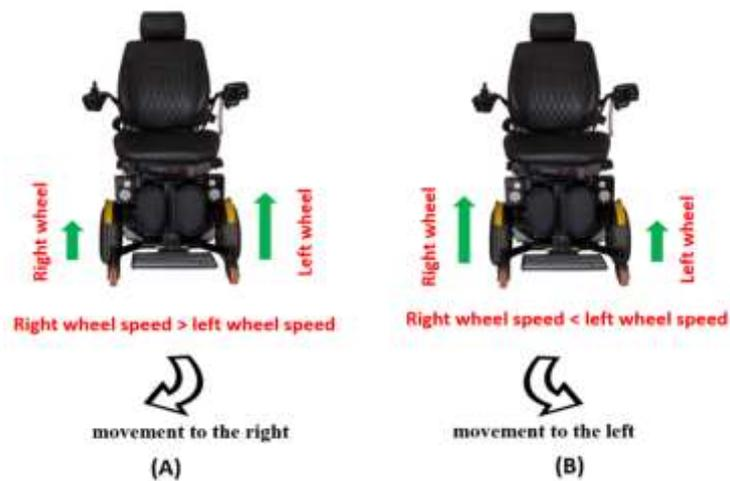
Figure 13 (A) Wheelchair movement to the right under the influence of acceleration sensor, (B) Wheelchair movement to the left under the influence of acceleration sensor
