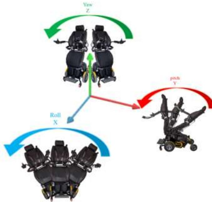
Figure 11 Axes for Euler angles definition for EWC
