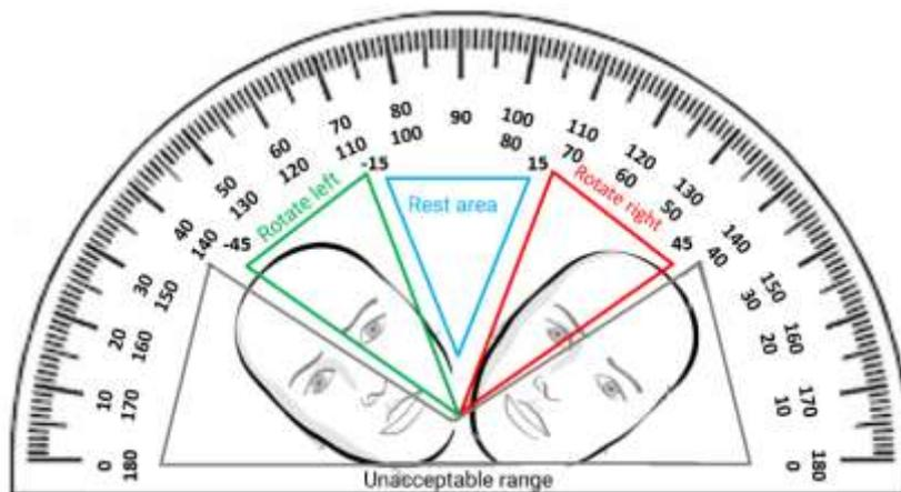
Figure 12 Motion threshold values in the acceleration sensor section around the Roll axis
