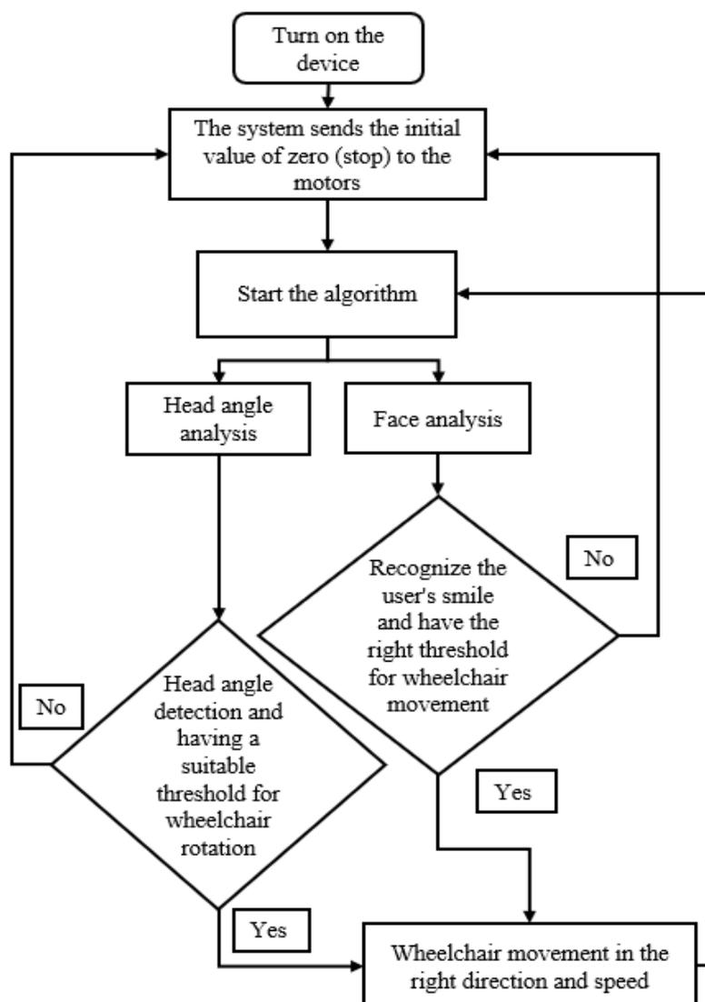
**Figure 6** Flowchart of the designed algorithm
