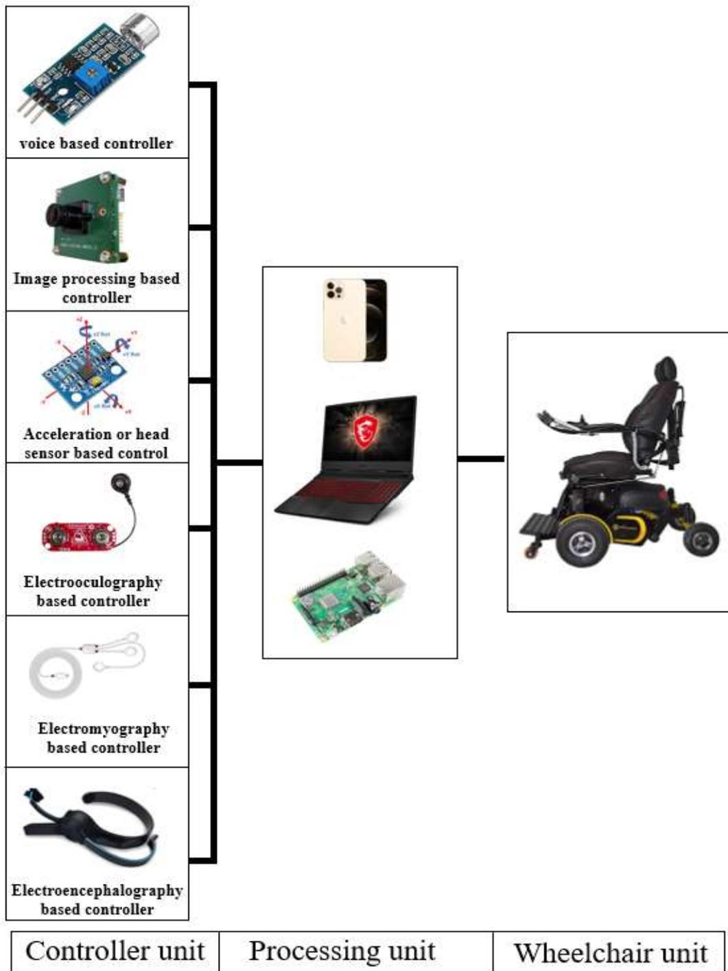
**Figure 1** Types of user-machine interactions for EWC movement control
