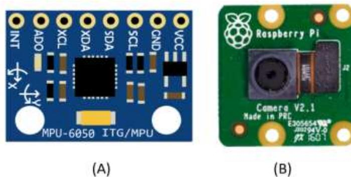
**Figure 3** (A) MPU6050 module, (B) Camera module
