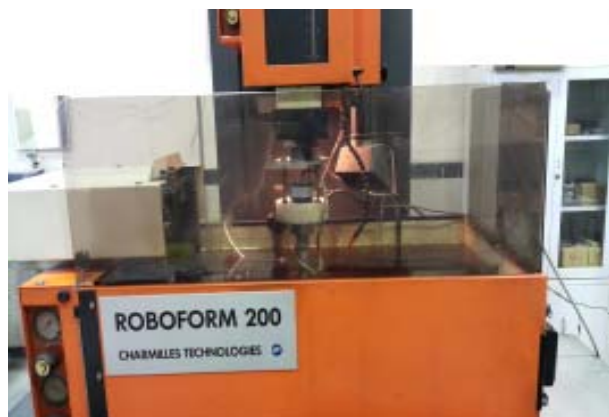
Figure 2 The spark machine which was used at ultrasonic vibrations assisted EDM
