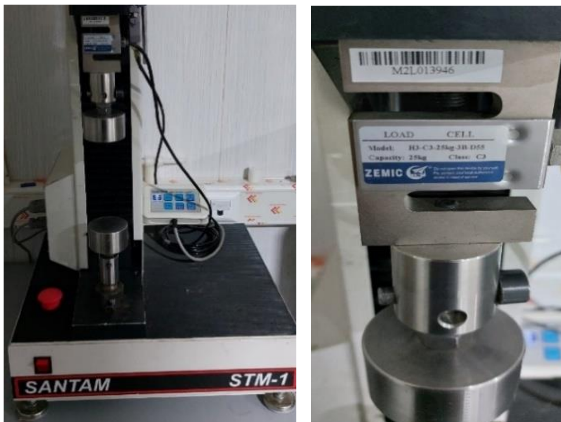
Figure 3 Device for the compression test (STM-1); the upper and lower plates are moving and fixed, respectively. The specimen is located on the fixed plate, and a uniaxial compression is applied to the sample with a controlled velocity.
