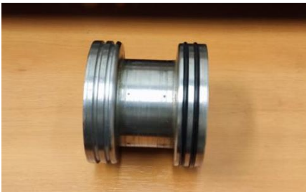
Figure 16 Porous piece of the air bearing with two rows of pores with a diameter of 0.2 mm
