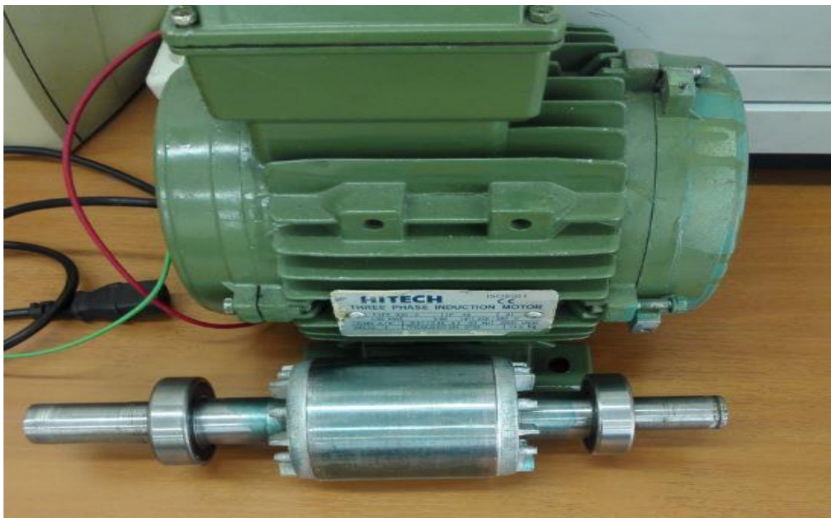
Figure 10 A 1.5kW three-phase induction motor and its dismantled rotor
