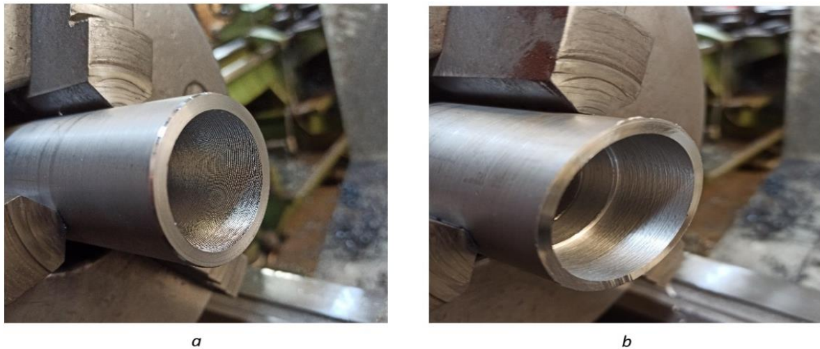
Figure 10 The surface quality of the workpiece with self-excited vibration (a) and without self-excited vibration (b)
