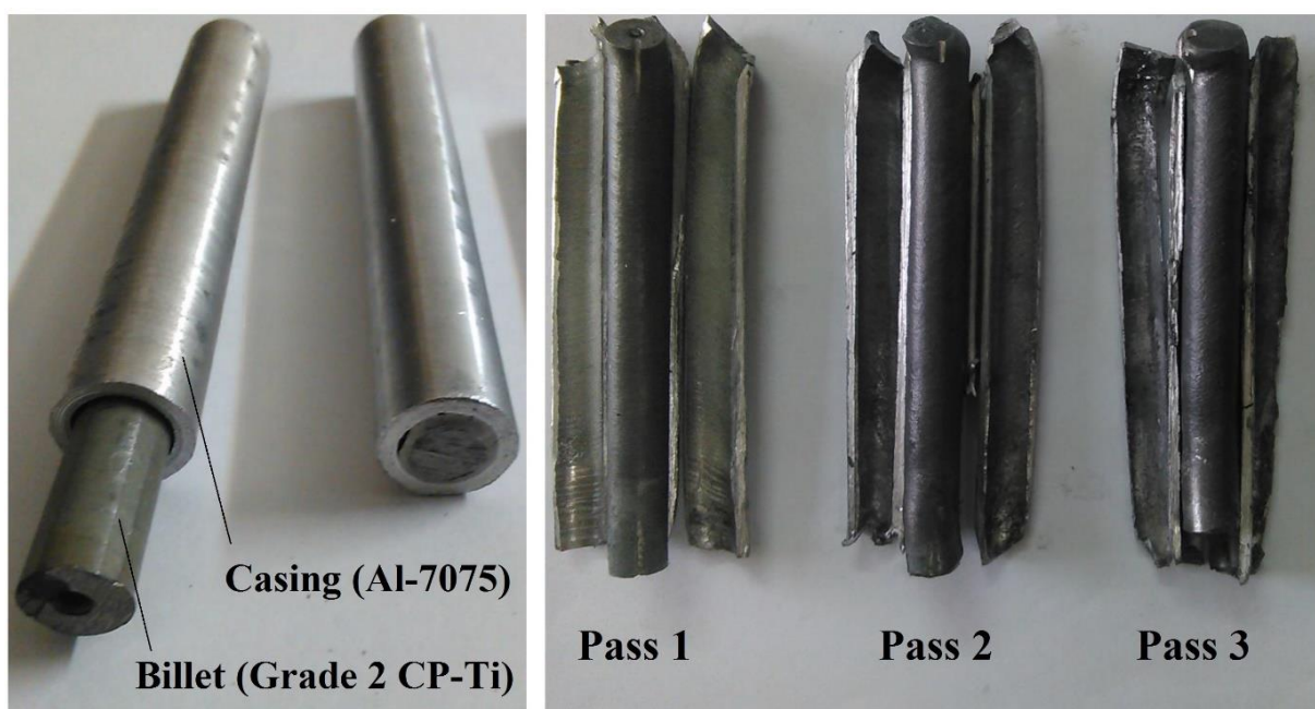
Figure 3 Bimetallic specimens, before and after 1 to 3 passes of ECAP
