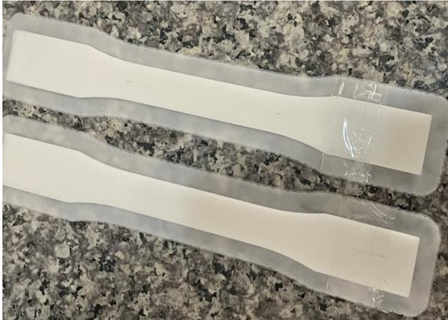
Figure 3 Stretch samples after printing in line pattern
