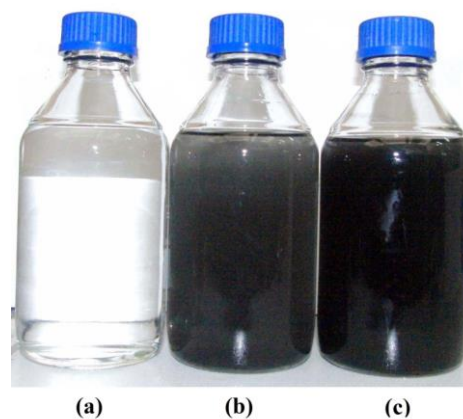
Figure 1 Working fluids (a) pure water, (b) 0.01 vol.%, and (c) 0.1 vol.% ferrofluid.
