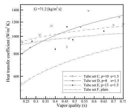
Figure 6 Variation of the heat transfer coefficient versus the vapor quality for coiled wire equipped and plain tubes of C, D, E, and F at G=71.2 [Kg/m<sup>2</sup>s]
