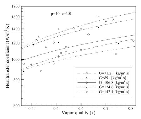
Figure 7 Variation of the heat transfer coefficient versus the vapor quality for different mass velocities in pipe B
