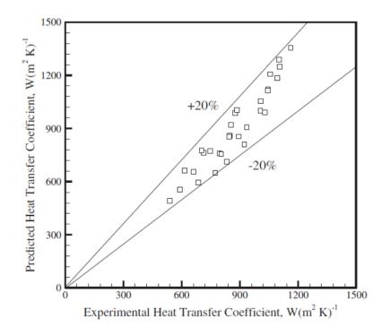
Figure 3 Comparison of the present heat transfer coefficients with the results of ref. [14]
