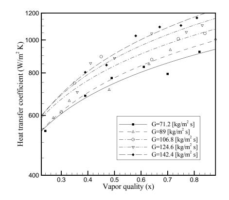
Figure 4 Variation of the heat transfer coefficient versus the vapor quality for different mass velocities
