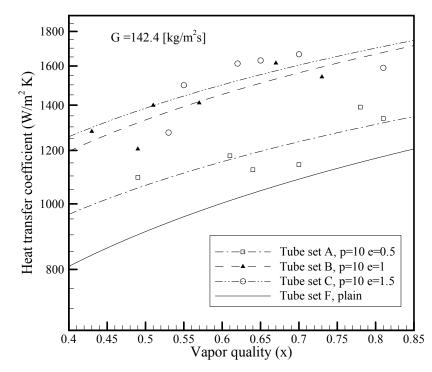
Figure 5 Variation of the heat transfer coefficient versus the vapor quality for coiled wire equipped and plain tubes of A, B, C, and F at G=142.4 [Kg/m<sup>2</sup>s]
