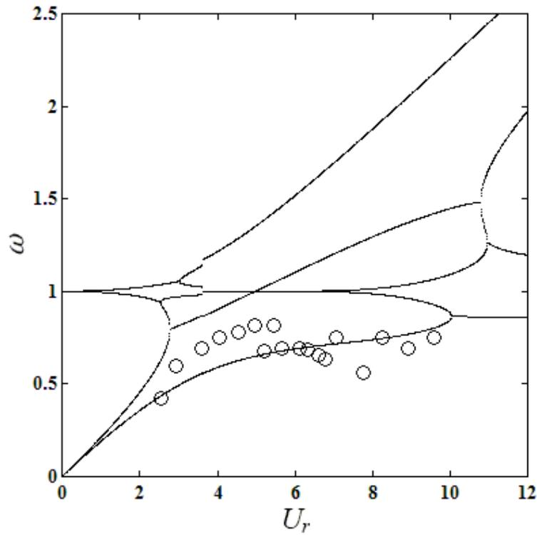
**Figure 9:** Frequency response of the modified model for low mass-damping ratio. —, modified model; ○, experimental data of Brankovic and Bearman [27] for  $m^*=0.83$ ,  $l=0.584$  m and  $\zeta=2.5 \times 10^{-4}$  ( $\mu=1.1661$ ).
