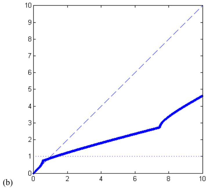
**Figure 5.** Effect of the flow velocity  $\Omega$  on the frequency of the dominant mode of the coupled system. (a)  $AM=0.05$ , the frequency deviates from Strouhal law only near  $\Omega=1$ , by coupled mode flutter.  $AM=0.75$  the frequency deviates from Strouhal law in a large range of coupled mode flutter, and also is affected outside this range. -, frequency; ..., uncoupled solution; W, wake mode; CMF, coupled mode flutter.
