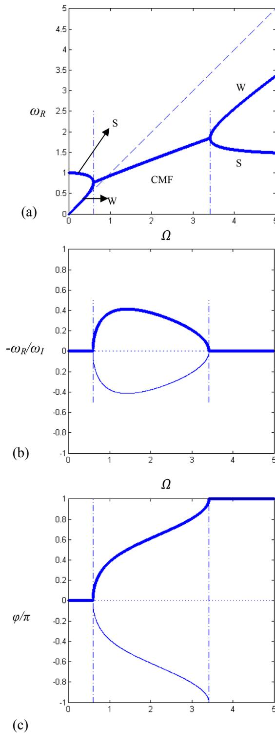
**Figure 2.** Effect of the dimensionless flow velocity  $\Omega$  on the modes of the coupled system defined by Eq. (12), for  $AM=0.5$ : (a) frequency, (b) growth rate (c) phase between the lift  $q$  and the displacement  $y$ . -, unstable mode; -, damped mode; --, limit of the lock-in range; ..., wake mode of uncoupled solution when  $AM=0$ . In (a), S denotes a structure mode, W denotes a wake mode and CMF is a coupled-mode flutter solution.
