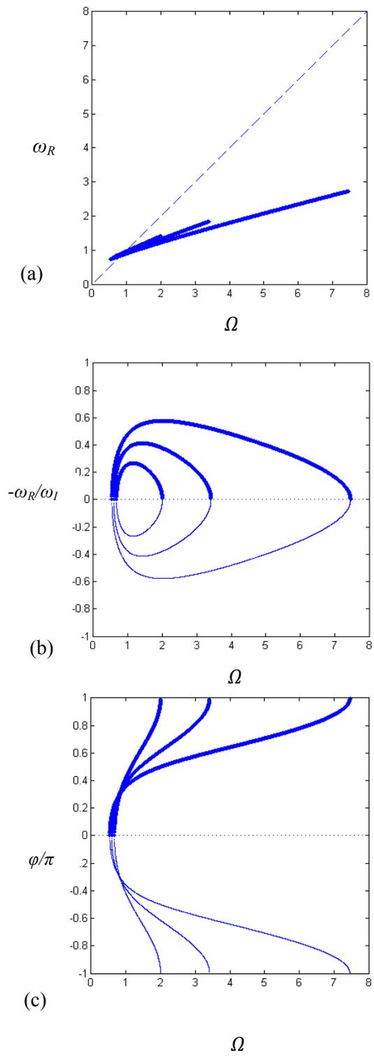
**Figure 3.** Influence of the combined mass parameter  $AM$  on the characteristics of lock-in: (a) frequency, (b) growth rate, (c) phase between the lift  $q$  and the displacement  $y$ . In each plot the results for three values of  $AM$  are shown, 0.25, 0.50 and 0.75. -, unstable mode; -, damped mode; -.-, ..., wake mode of the uncoupled solution when  $AM=0$ .
