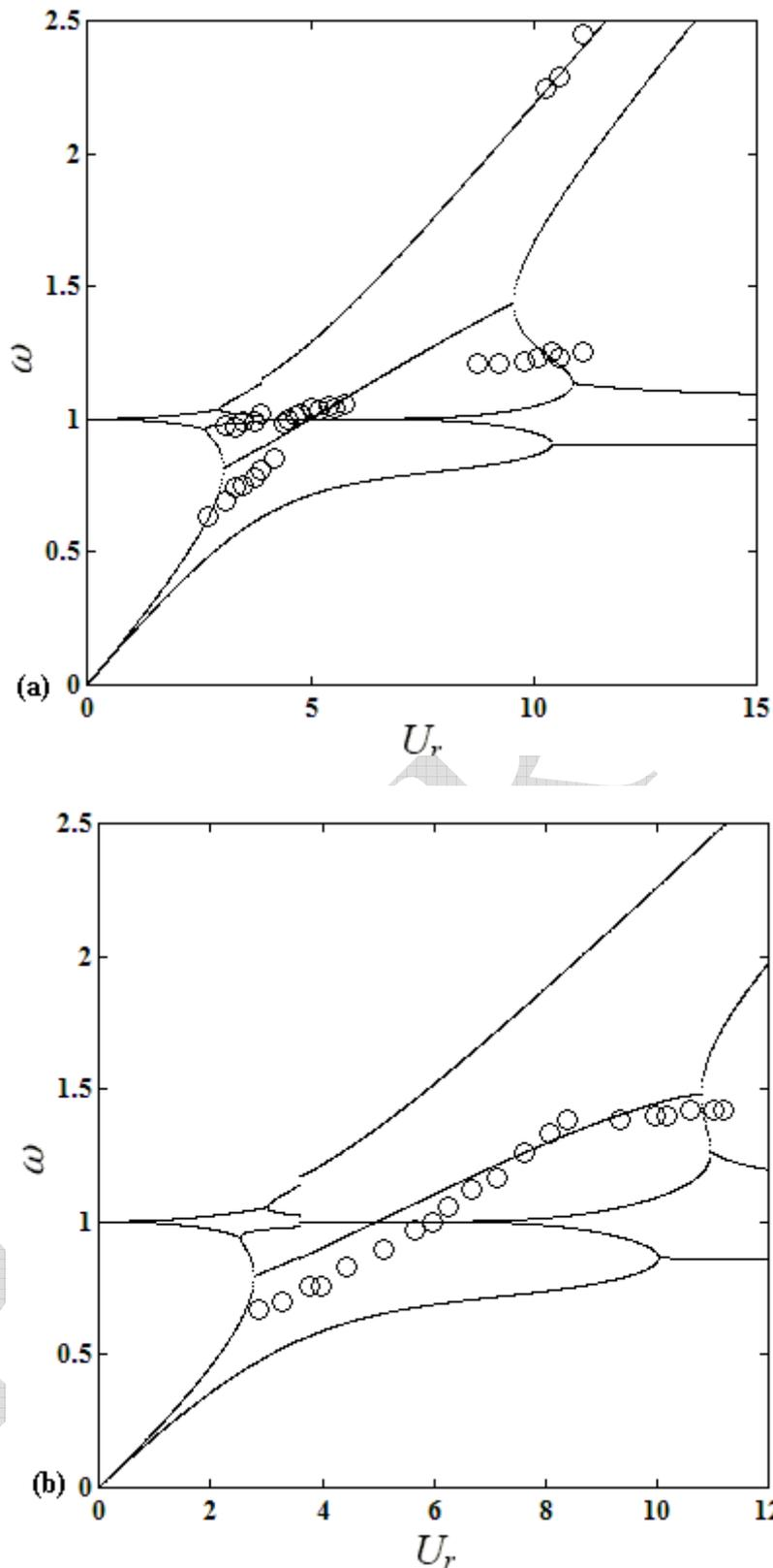
**Figure 8:** Frequency response of the modified model for low mass-damping ratio. (a) —, modified model;  $\circ$ , experimental data of Williamson and Khakak [9] for  $m^* = 3.3$ ,  $l = 0.381$  m and  $\zeta = 0.0026$  ( $\mu = 1.773$ ). (b) —, modified model;  $\circ$ , experimental data of Brankovic and Bearman [27] for  $m^* = 0.82$ ,  $l = 0.584$  m and  $\zeta = 1.5 \times 10^{-4}$  ( $\mu = 1.1615$ ).
