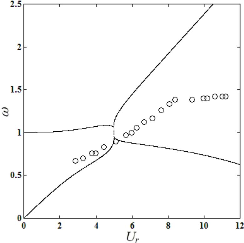
**Figure 7:** Frequency response of the classical model for low mass-damping ratio ( $\mu=1.1615$ ,  $\xi=1.5 \times 10^{-4}$ ). —, the classical wake oscillator model;  $\circ$ , Branković and Bearman’s experimental results [27].
