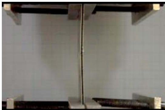
Figure 8 FML plates with 10mm opening on the verge of buckling (point A)
