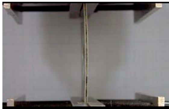
Figure 14 FML plates with 20mm opening on the verge of buckling (point A)
