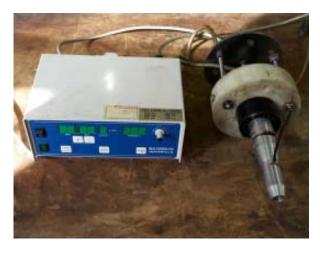
Figure 1 The ultrasonic vibration generator
